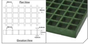
Section Properties per m of Width: A = 4.57x103mm<sup>2</sup> I=4.37x10<sup>5</sup>mm<sup>4</sup> S=2.58x10<sup>4</sup>mm<sup>3</sup> \*Not available with meniscus top surface (only grit)
