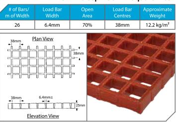
Section Properties per m of Width:  $A = 3.62 \times 103 \text{mm}^2$   $I = 1.91 \times 10^5 \text{mm}^4$   $S = 1.56 \times 10^4 \text{mm}^3$
