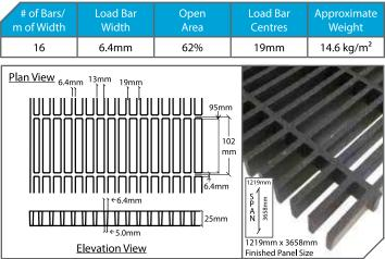
Section Properties per m of Width: A = 7.58x103mm<sup>2</sup> I = 4.07x10<sup>5</sup>mm<sup>4</sup> S = 308x10<sup>4</sup>mm<sup>3</sup>
