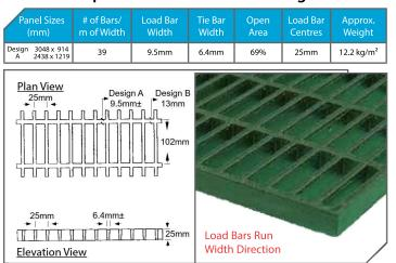
$\underline{Section\ Properties\ per\ m\ of\ Width}:\ A=5.44x103mm^2\ \ I=3.00x10^5mm^4\ \ S=2.31x10^4mm^3$
