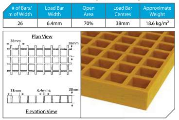
Section Properties per m of Width: A = 6.03x103mm<sup>2</sup> I = 6.96x10<sup>5</sup>mm<sup>4</sup> S= 3.49x10<sup>4</sup>mm<sup>3</sup>
