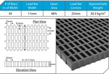
Section Properties per m of Width: A = 1.58x10<sup>4</sup>mm<sup>2</sup> I = 1.90x10<sup>6</sup>mm<sup>4</sup> S= 9.68x10<sup>4</sup>mm<sup>4</sup>
