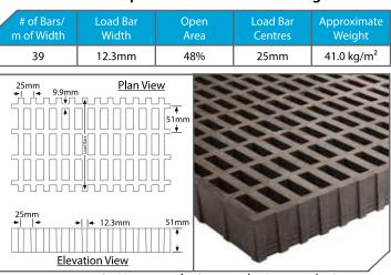
Section Properties per m of Width: A = 2.17x10<sup>4</sup>mm<sup>2</sup> I = 1.83x10<sup>5</sup>mm<sup>4</sup> S = 1.76x10<sup>5</sup>mm<sup>3</sup>
