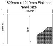
Note: Load carrying bars are oriented across the narrow (1219mm) dimension of the panel. Panels furnished with closed bars all sides.
